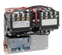
Reversing motor starter Size 0 Three phase full voltage Solid-state overload relay OLRelay amp range 0.75-3.4A 24Vdc coil Non-combination type Enclosure type (open)
