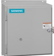
Reversing motor starter, Size 3 1/2, Three phase full voltage, Solid-state overload relay, OLR amp range 50-200A, 208VAC 60Hz coil, Non-combination type, Enclosure type 4X fiberglass, Water/dust tight noncorrosive, Standard width enclosure
