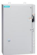
Non-reversing motor starter, Size 2 1/2, Three phase full voltage, Solid-state overload relay, OLR amp range 25-100A, Combination type, 100A fusible disconnect, 100A/250V fuse clip, Enclosure NEMA type 4/12, Water/dust tight for outdoors, Extra-wide enclosure
