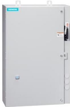
Non-reversing motor starter Size 4 Three phase full voltage Solid-state overload relay OLRelay amp range 50-200A 208VAC 60HZ coil Combination type 150A circuit breaker Enclosure NEMA type 4/12 Water/dust tight for outdoors Standard width enclosure
