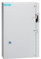
Non-reversing motor starter, Size 2 1/2, Three phase full voltage, Solid-state overload relay, OLR amp range 25-100A, Combination type, 100A fusible disconnect, 100A/600V fuse clip, Enclosure NEMA type 1, Indoor general purpose use, Extra-wide enclosure
