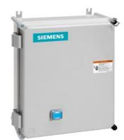
Non-reversing motor starter, Size 0, Three phase full voltage, Solid-state overload relay, OLR amp range 3-12A, Non-combination type, Enclosure type 4X fiberglass, Water/dust tight noncorrosive, Standard width enclosure
