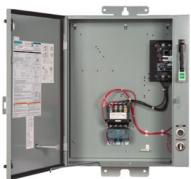
Pump control panel, Size 1, Three phase full voltage, Solid-state overload relay, OLR amp range 5.5-22A, 380-440/440-480V 50/60Hz coil, Standard type contactor, 25A circuit breaker, HOA Sel Sw. <(>&<)> Start P.B., Enclosure NEMA type 3/3R, Weather proof outdoor use
