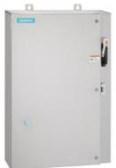
Non-reversing motor starter, Size 2 1/2, Three phase full voltage, Solid-state overload relay, OLR amp range 25-100A, 24VDC coil, Combination type, 100A fusible disconnect, 100A/250V fuse clip, Encl NEMA type 4X 304 S-Steel, Water/dust tight noncorrosive, Extra-wide enclosure
