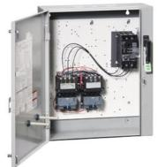
2-speed 3-phase motor starter, Size 1, Two separate windings, Constant or variable torque, Solid-state overload relays, Low Spd OLR range 10-40A, High Spd OLR range 10-40A, 110V 50Hz / 120V 60Hz coil, Combination type, 30A circuit breaker, Enclosure NEMA type 4/12, Water/dust tight for outdoors
