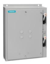
Duplex starter w/o alternator Size 3.5 Three phase full voltage Solid-state overload relay OLR amp range 50-200A 110VAC 50Hz / 120VAC 60Hz Coil Combination type Two 200A disconnect switches Enclosure NEMA type 4/12 Water/dust tight weather proof
