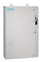
Non-reversing motor starter Size 1 Three phase full voltage Solid-state overload relay OLRelay amp range 3-12A 208VAC 60HZ coil Combination type 30Amp non-fusible disconnect Encl NEMA type 4X 316 S-steel Water/dust tight non-corrosive Extra-wide enclosure
