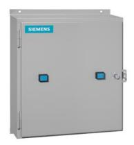
Duplex starter w/o alternator, Size 3 1/2, Three phase full voltage, Solid-state overload relay, OLR amp range 50-200A, 190-220/220-240V 50/60Hz coil, Noncombination type, Encl NEMA type 4X 304 S-Steel, Water/dust tight noncorrosive
