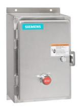
Non-reversing motor starter Size 1 Three phase full voltage Solid-state overload relay OLRelay amp range 3-12A 110VAC 50HZ / 120VAC 60HZ coil Non-combination type Encl NEMA type 4X 316 S-steel Water/dust tight non-corrosive Standard width enclosure
