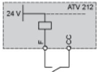
“PLC” position with PLC transistor outputs
