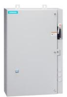
Non-reversing motor starter, Size 2, Three phase full voltage, Solid-state overload relay, OLR amp range 13-52A, 240V 50Hz / 277V 60Hz coil, Combination type, 50A circuit breaker, Encl NEMA type 4X 304 S-Steel, Water/dust tight noncorrosive, Extra-wide enclosure
