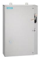
Non-reversing motor starter Size 0 Three phase full voltage Solid-state overload relay OLRelay amp range 0.75-3.4A 110VAC 50HZ / 120VAC 60HZ coil Combination type 30Amp non-fusible disconnect Encl NEMA type 4X 316 S-steel Water/dust tight non-corrosive Extra-wide enclosure
