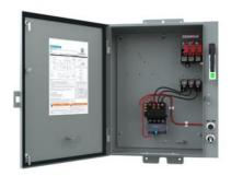
Pump control panel, Size 1 3/4, Three phase full voltage, Solid-state overload relay, OLR amp range 10-40A, 110-120/220-240VAC 60Hz coil, Standard type contactor, 30A fusible disconnect, 30A/600V fuse clip, HOA Sel Sw. <(>&<)> Start P.B., Enclosure NEMA type 3/3R, Weather proof outdoor use
