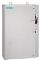
Non-reversing motor starter Size 0 Three phase full voltage Solid-state overload relay OLRelay amp range 5.5-22A Combination type 30Amp non-fusible disconnect Encl NEMA type 4X 316 S-steel Water/dust tight non-corrosive Extrawide enclosure
