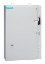
Non-reversing motor starter, Size 0, Three phase full voltage, Solid-state overload relay, OLR amp range 5.5-22A, 24VDC coil, Combination type, 30A non-fusible disconnect, Encl NEMA type 4X 304 S-Steel, Water/dust tight noncorrosive, Extrawide enclosure
