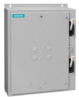
Duplex starter w/o alternator Size 0 Three phase full voltage Solid-state overload relay OLR amp range 3-12A 24VAC 50-60Hz Coil Combination type Two 30A disconnect switches Encl NEMA type 4X 304 S. Steel Water/dust tight non-corrosive
