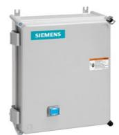
Non-reversing motor starter, Size 1, Three phase full voltage, Solid-state overload relay, OLR amp range 0.75-3.4A, Non-combination type, Enclosure type 4X fiberglass, Water/dust tight noncorrosive, Standard width enclosure
