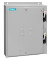
Duplex starter w/o alternator, Size 0, Three phase full voltage, Solid-state overload relay, OLR amp range 0.25-1A, 380-440/440-480V 50/60Hz coil, Combination type, Two 3A circuit breakers, Enclosure NEMA type 12, Dust/drip proof for indoors
