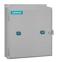
Duplex starter w/o alternator, Size 0, Three phase full voltage, Solid-state overload relay, OLR amp range 0.25-1A, 208VAC 60Hz coil, Non-combination type, Encl NEMA type 4X 304 S-Steel, Water/dust tight noncorrosive
