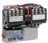
Reversing motor starter Size 0 Three phase full voltage Solid-state overload relay OLRelay amp range 0.25-1A 550/575-600 50/60HZ coil Non-combination type Enclosure type (open)
