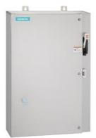
Non-reversing motor starter Size 3 Three phase full voltage Solid-state overload relay OLRelay amp range 25-100A 208VAC 60HZ coil Combination type 100A non-fusible disconnect Encl NEMA type 4X 316 S-steel Water/dust tight non-corrosive Extra-wide enclosure
