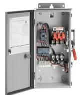
Slim Line Pump Control Panel NEMA size 1 Three phase full voltage Solid-state overload relay OLR amp range 5.5-22A 460VAC 60Hz Coil 30A fusible disconnect 30A/600V fuse clip 1NC / 1NO auxiliary contacts HOA Sel. Sw. <(>&<)> Start/Stop 3-point power terminal block 3-point control terminal block 3-point ground lug Enclosure NEMA type 3/3R Weather proof outdoor use
