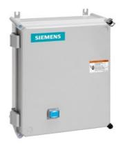
Non-reversing motor starter, Size 1, Three phase full voltage, Solid-state overload relay, OLR amp range 3-12A, 208VAC 60Hz coil, Non-combination type, Enclosure type 4X fiberglass, Water/dust tight noncorrosive, Standard width enclosure
