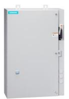
Non-reversing motor starter, Size 3, Three phase full voltage, Solid-state overload relay, OLR amp range 25-100A, Combination type, 200A fusible disconnect, 200A/250V fuse clip, Enclosure NEMA type 4/12, Water/dust tight for outdoors, Standard width enclosure
