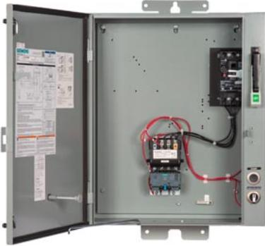
Pump control panel, Size 1, Three phase full voltage, Solid-state overload relay, OLR amp range 10-40A, 110-120/220-240VAC 60Hz coil, Standard type contactor, 30A circuit breaker, HOA Sel Sw. Start P.B., Enclosure NEMA type 3/3R, Weather proof outdoor use
