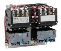
2-speed 3-phase motor starter Size 3 One winding consequent pole Constant horsepower Solid-state overload relays Low SPD OLR range 13-52a High SPD OLR range 25-100A 110V 50HZ / 120V 60HZ coil Enclosure NEMA type (open) No enclosure
