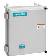
Non-reversing motor starter, Size 1, Three phase full voltage, Solid-state overload relay, OLR amp range 0.25-1A, Non-combination type, Enclosure type 4X fiberglass, Water/dust tight noncorrosive, Standard width enclosure
