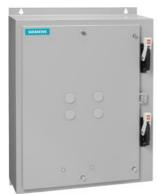
Pump control panel, Duplex controller NEMA size 0 Solid-state overload relay, OLR amp range 3-12A, 120 VAC coil, Fusible disconnect HOA Sel Sw. and Start P.B., Enclosure NEMA type 3/3R,12 Weather proof outdoor use
