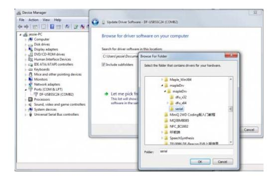
5) Reset Veyron Servo Driver 24-Channel with RET button, wait for the blue light stops flashing. At this point Windows will prompt to install the driver, too. Please manually locate the directory, select mapleDrv -->serial in the folder. Until now, the driver has been installed
