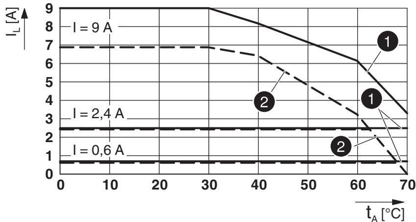
Figure 7 Derating curve
