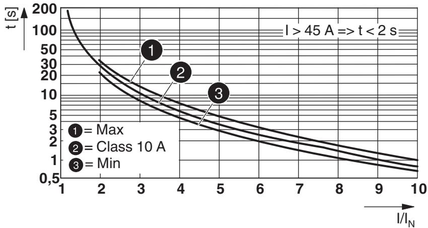
Figure 6 Trigger characteristic
