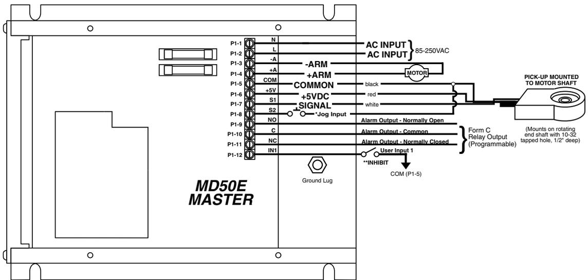
\* For AC inputs utilizing two hot lines, both inputs should be protected with appropriately sized fuses or circuit breakers.
