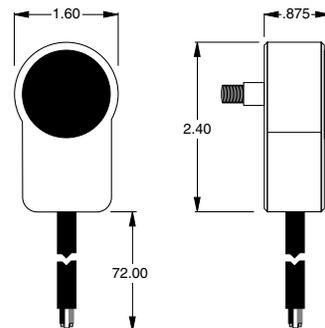
No other mounting screws are necessary, as the cord will keep the unit from rotating.
