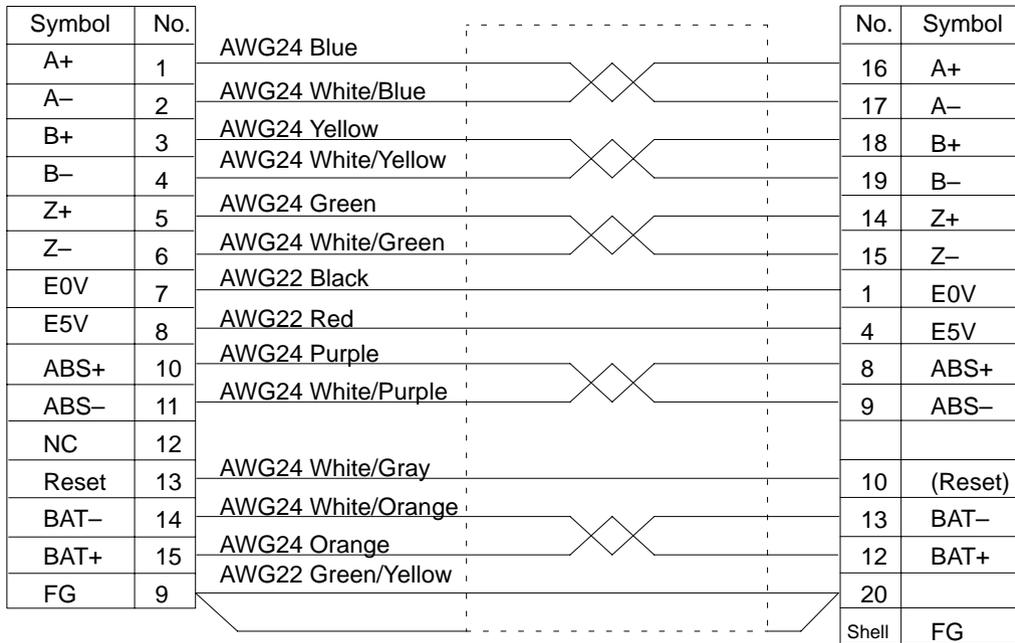
Cable: AWG22 × 3C + AWG24 × 6P
