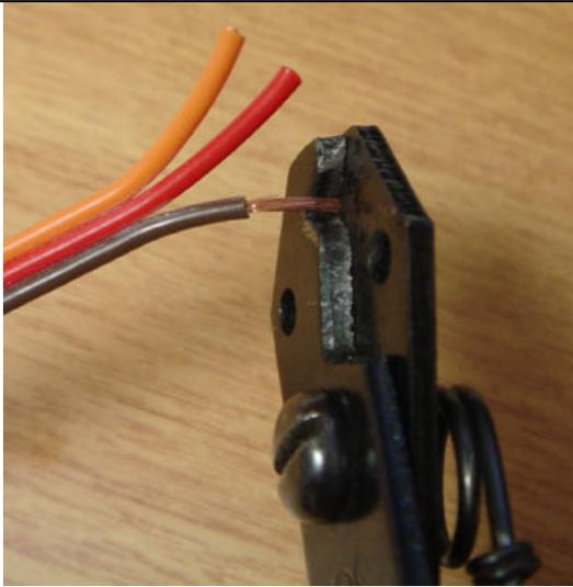
**Step 1:** Strip the wire which you are using approximately 1/4". The wires may be 14 gauge to 30 gauge
