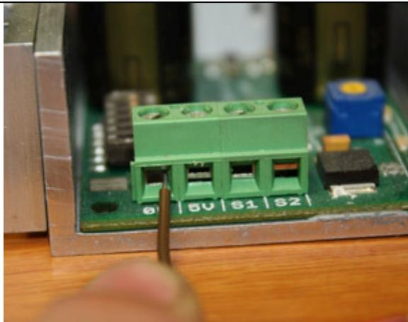
**Step 3:** Insert the stripped portion of the wire into the opening in the screw terminal
