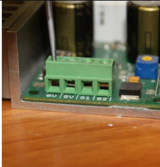
**Step 2:** With a small screwdriver, turn the top screw counter-clockwise until it stops gently.
