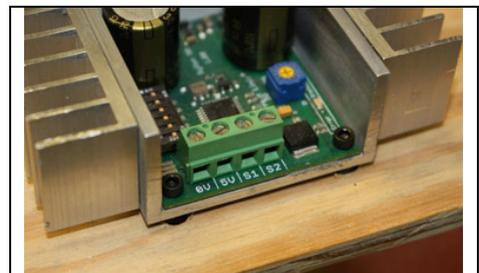
Figure 2.3: Mounted to a wood frame using standoffs
