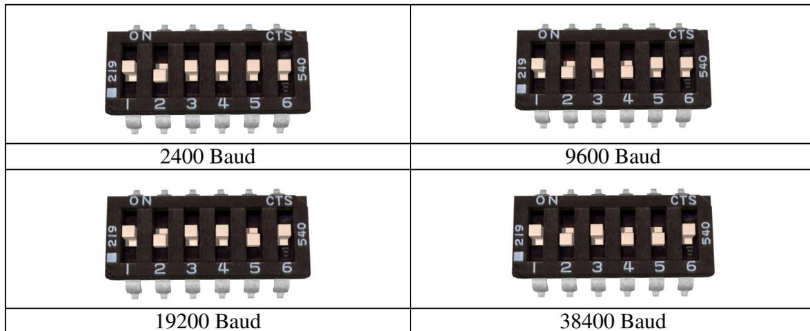
What baud rate to use is dependent on what your host can provide and the update speed necessary. 9600 baud or 19200 baud are recommended as the best starting points. If communication is unreliable, decrease the baud rate. If communications are reliable, you may increase the baud rate. The maximum update speed on the SyRen 50 is approximately 2000 commands per second. Sending characters faster than this will not cause problems, but it will not increase the responsiveness of the controller either.
