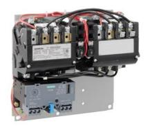
Reversing motor starter Size 0 Three phase full voltage Solid-state overload relay OLRelay amp range 3-12A 110VAC 50HZ / 120VAC 60HZ coil Non-combination type Enclosure type (open)
