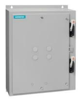
Duplex starter w/o alternator, Size 0, Three phase full voltage, Solid-state overload relay, OLR amp range 5.5-22A, 110V 50Hz / 120V 60Hz coil, Combination type, Two 25A circuit breakers, Encl NEMA type 4X 304 S-Steel, Water/dust tight noncorrosive
