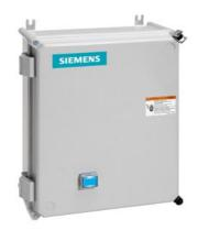
Non-reversing motor starter, Size 1, Single phase full voltage, Solid-state overload relay, OLR amp range 5.5-22A, 110V 50Hz / 120V 60Hz coil, Non-combination type, Enclosure type 4X fiberglass, Water/dust tight noncorrosive, Standard width enclosure
