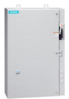
Non-reversing motor starter, Size 3, Three phase full voltage, Solid-state overload relay, OLR amp range 25-100A, Combination type, 100A fusible disconnect, 100A/250V fuse clip, Enclosure NEMA type 4/12, Water/dust tight for outdoors, Extra-wide enclosure
