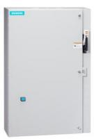
Non-reversing motor starter, Size 3, Three phase full voltage, Solid-state overload relay, OLR amp range 25-100A, Combination type, 100A non-fusible disconnect, Enclosure NEMA type 1, Indoor general purpose use, Extra-wide enclosure
