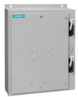
Duplex starter w/o alternator Size 2 Three phase full voltage Solid-state overload relay OLR amp range 13-52A Combination type Two 60A disconnect switches Enclosure NEMA type 4/12 Water/dust tight weather proof
