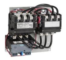
Reversing motor starter Size 4 Three phase full voltage Solid-state overload relay OLRelay amp range 50-200A 110-120/220-240VAC 60HZ coil Non-combination type Enclosure type (open)
