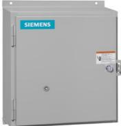
Reversing motor starter, Size 3 1/2, Three phase full voltage, Solid-state overload relay, OLR amp range 50-200A, Non-combination type, Enclosure type 4X fiberglass, Water/dust tight noncorrosive, Standard width enclosure
