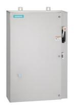
Non-reversing motor starter Size 1 3/4 Three phase full voltage Solid-state overload relay OLRelay amp range 10-40a Combination type 60Amp non-fused disconnect Encl NEMA type 4X 316 S-steel Water/dust tight non-corrosive Extrawide enclosure
