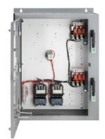
Duplex starter with alternator Size 1 Three phase full voltage Solid-state overload relay OLR amp range 10-40A 110VAC 50Hz / 120VAC 60Hz Coil Combination type Two 30A disconnect switches Encl NEMA type 4 painted steel Water/dust tight weather proof
