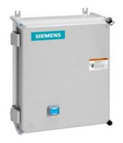
Non-reversing motor starter, Size 1, Single phase full voltage, Solid-state overload relay, OLR amp range 5.5-22A, 24VDC coil, Non-combination type, Enclosure type 4X fiberglass, Water/dust tight noncorrosive, Standard width enclosure
