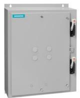
Duplex starter w/o alternator Size 0 Three phase full voltage Solid-state overload relay OLR amp range 0.75-3.4A 24VAC 50-60Hz Coil Combination type Two 30A disconnect switches Encl NEMA type 4 painted steel Water/dust tight weather proof
