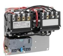
Reversing motor starter Size 1 Three phase full voltage Solid-state overload relay OLRelay amp range 0.75-3.4A 220-240/440-480VAC 60HZ coil Non-combination type Enclosure type (open)
